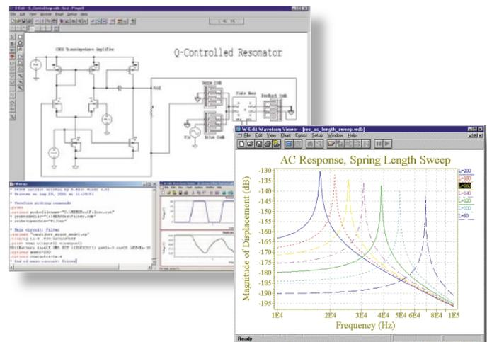
**Modeling Tools:** MEMS Modeler automatically generates behavioral models ready for system simulation with electronics and packaging from 3D data from finite element analysis programs. Complex, finite element models involving a large number of degrees of freedom are reduced to behavioral models with a few master degrees of freedom. Users can also create their own models from analytical equations and the tool generates simulation-ready descriptions in a variety of popular formats.
